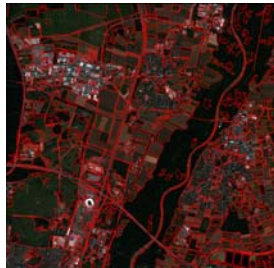
Figure 1 Automatic vector segmentation. The borders of the objects were smoothed in order to simplify the corresponding shape file.
