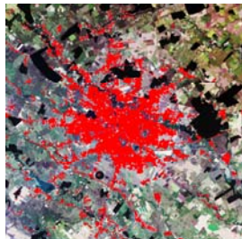
Figure 3 Bucharest scene segmentation. The red area is a collection of extracted objects. The collecting effort is an automatic process based on a machine learning algorithm.
